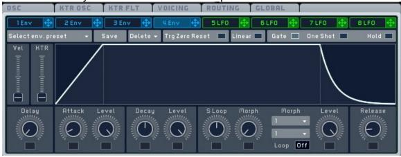
The funky parallelogram-looking thing in the middle is a visual representation of the dynamics of your sound. The linear slope on the left is the "attack," which controls the dynamics of the initial sound, the flat part at the top is the "decay," or what's happening to the sound while you are playing, and the last concave slope is the "release," or what happens to the sound after we stop generating it.
