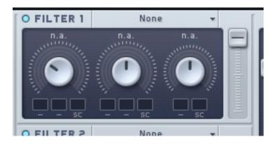
Select "Lowpass 2." Blow the EWI. See how the sound is now muffled? If we can assign the breath control to ramp up the cutoff dial a bit when we blow harder, not only will our sound get louder, but now it will get brighter, too. This is what happens when we play woodwind instruments, so it is only natural to make our synths behave the same way.
